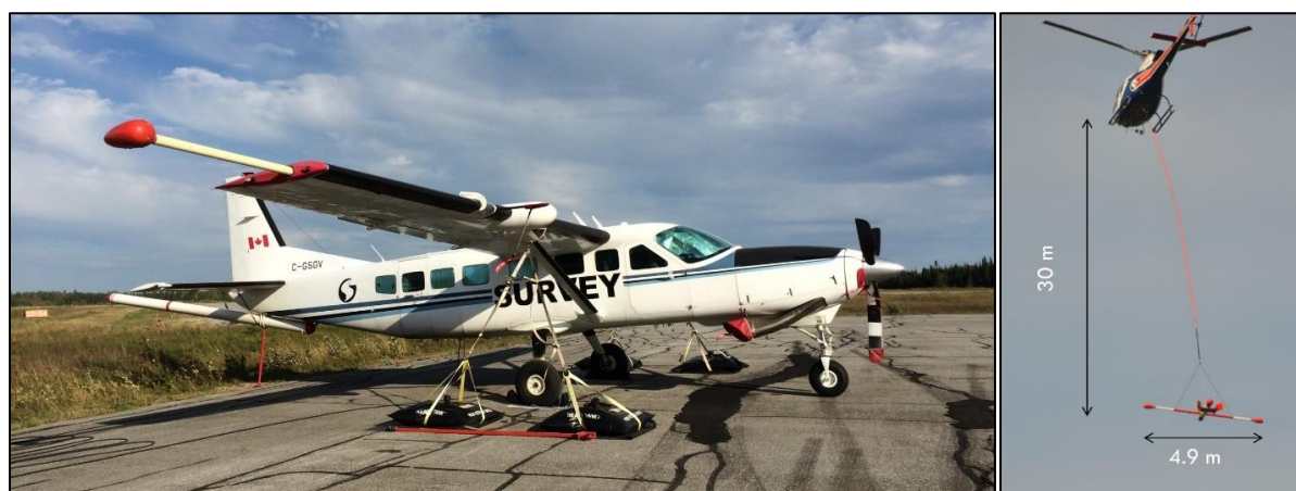
Figure 2. A fixed wing magnetic gradiometry system (left) with sensors located in tail and at each wing tip and a towed helicopter (right) system with two laterally spaced magnetic sensors.
